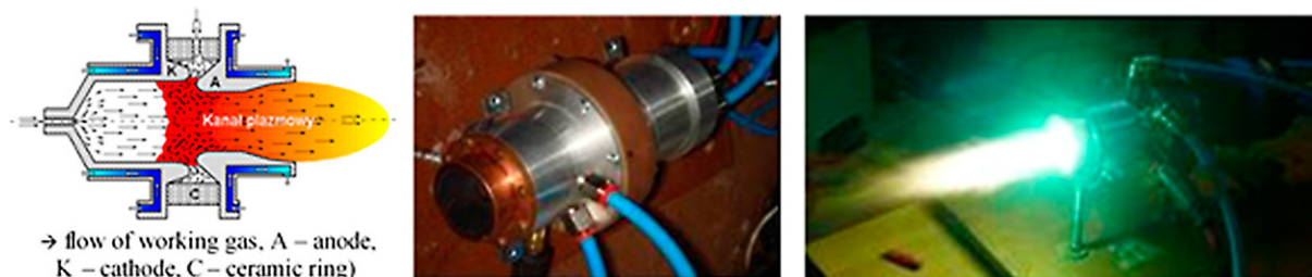
Fig. 1. Model and actual cavity plasmatron of PW type on test stand (operating power 12–28 kW) [4]
