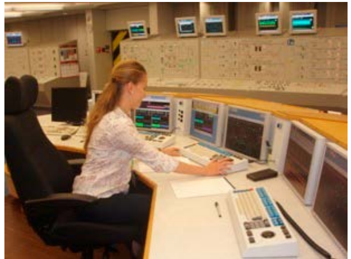
Fig. 6. Simulator of control room
