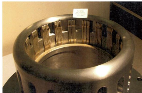
Photo 2: Main contact on fixed contact side
