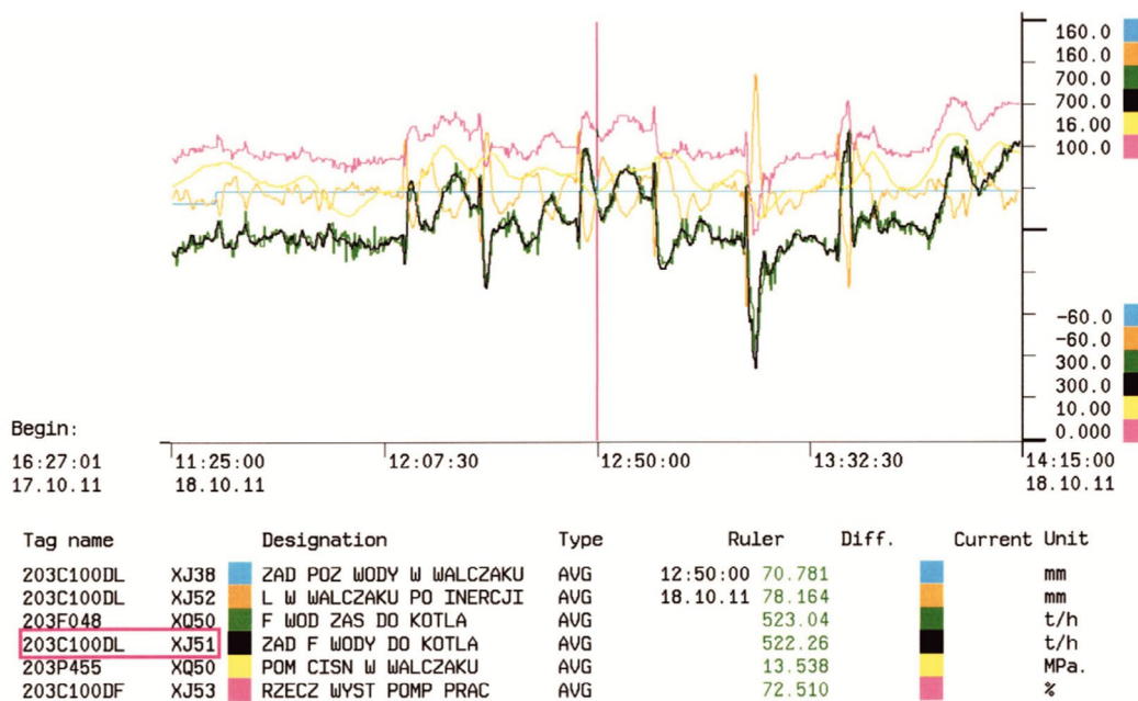
Figure 7. Response of 200 MW unit to primary control – comparison between “boiler follow” and “turbine follow” modes – operation of automatic control system for water level in boiler drum (set point – blue, real value – orange)
