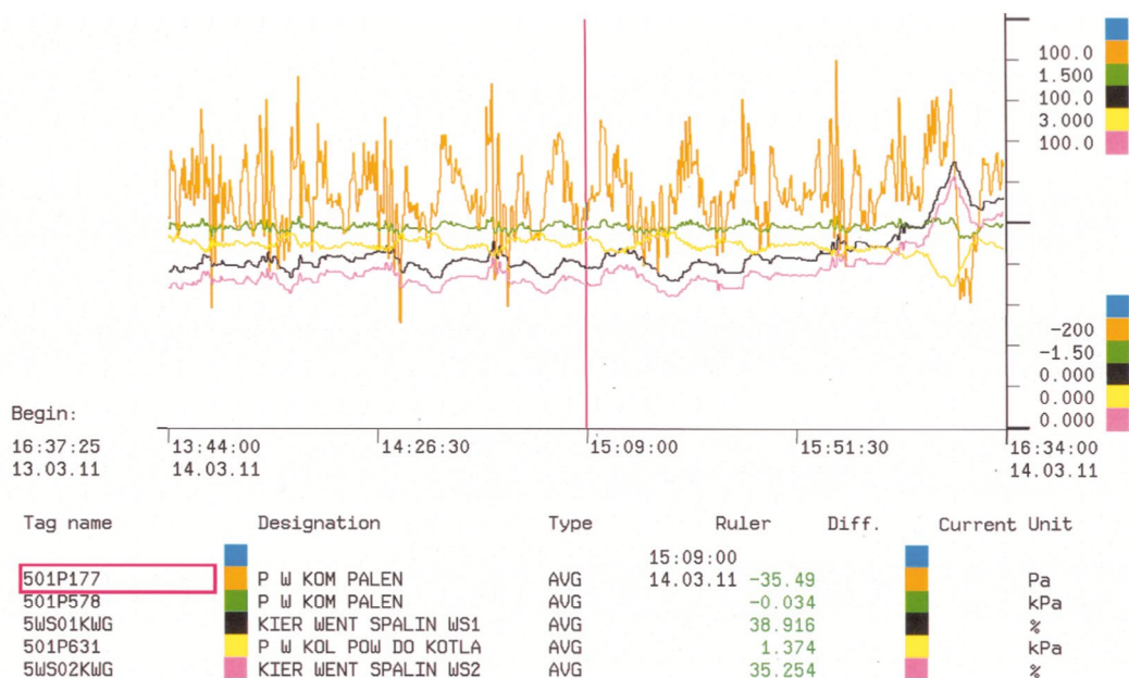
Figure 12. Response of 200 MW unit to secondary control – comparison between “boiler follow” and “turbine follow” modes – operation of automatic control circuit of pressure in furnace chamber (set point – green, real value – orange)
